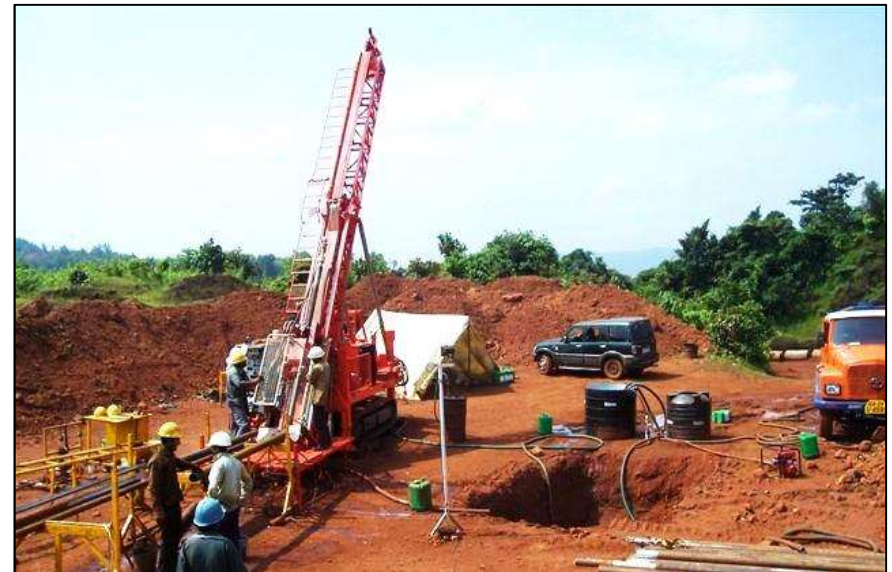
Exploration: Advanced Wireline Diamond Core Drilling
