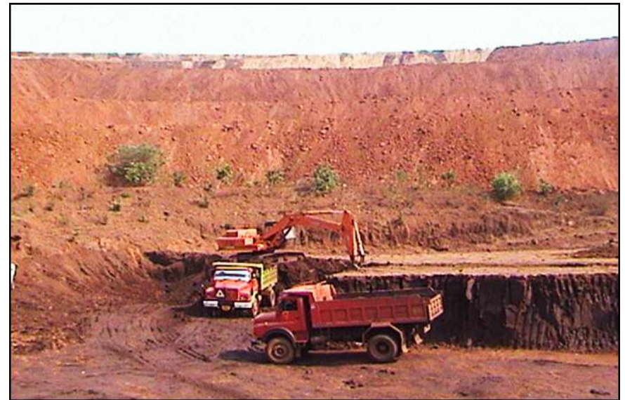
Monsoon Preparations: De-silting of Garland Drains & Settling Ponds
