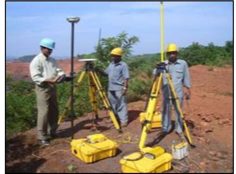
Utilization of Advances Mine Survey Equipments (Total Station, 3D Laser Scanner & DGPS)
