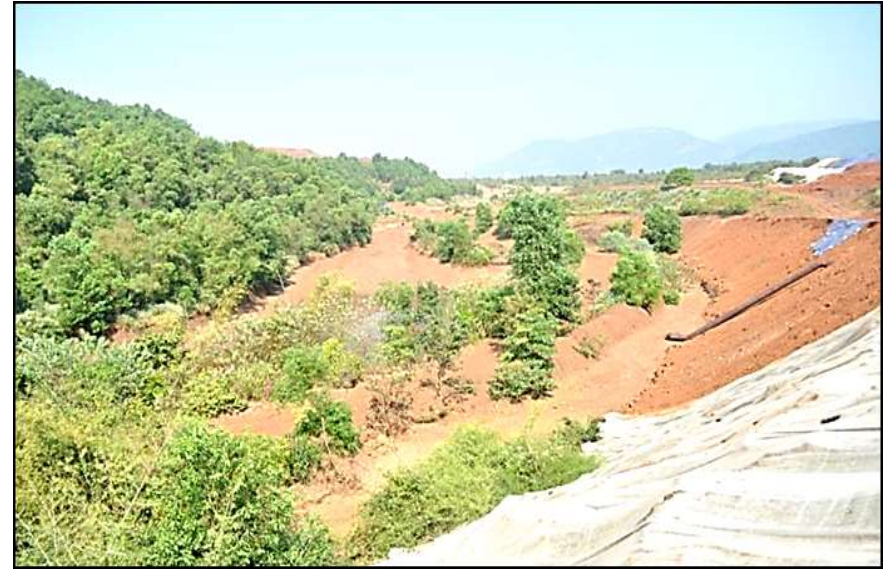
Environment Management: Provision of Garland Drains at the Dump Toe
